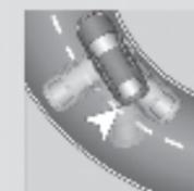
The application of the brake induces a force (arrow) that acts in the opposite direction of the slide, returning the car to its correct path.
