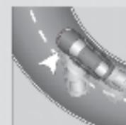
As the rear slides first in oversteer there is more grip available from the front tyres. ESP detects this and applies either the left or right (arrow) front brake.
